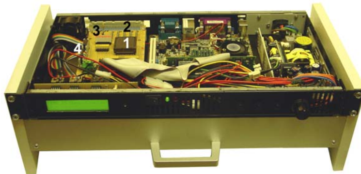
Fig. 1. A low-cost industrial PC based on a Mini-ITX motherboard. 1 - CPLD containing the ATA i/o adapter circuitry; 2 - interface connector; 3 - diagnostic LEDs; 4 - front-panel I/O attachment.
