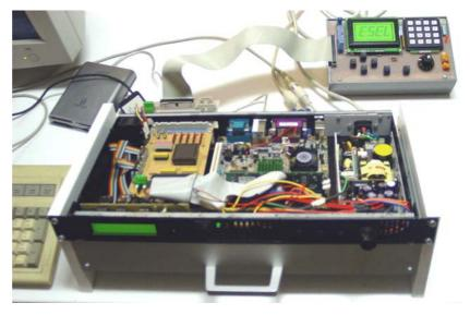
The cute small PC case contains a NanoITX motherboard and a GPIO ATA adapter connected to a makeshift experimental platform.
