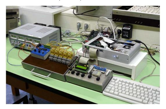
A closer look at the GPIO adapter (left) and the motherboard (right).
