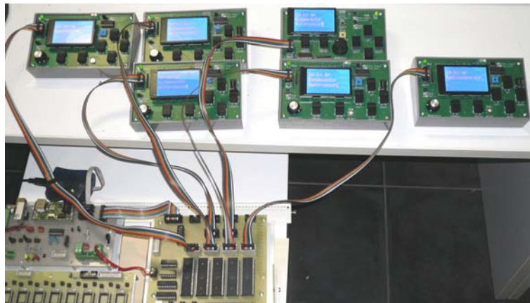
Fig. 3 To facilitate the bring-up of a complicated experimental multimicrocontroller system, each of the microcontrollers is connected to its own debugging console.
