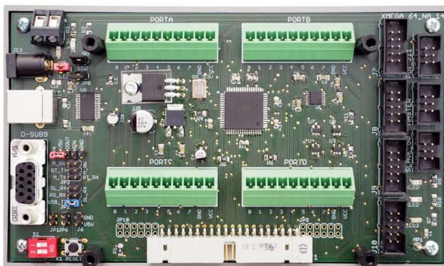
The photos show the first prototype (V1). Further development led to omitting the RS-232 signalization, reducing the number of jumpers to two, and changing the USB connector to mini-B.
