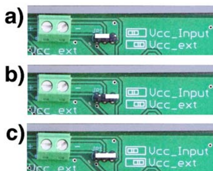
Fig. 5 Power supply jumper settings. a) Module powered by upstream device. b) Module powered via power-supply connectors. c) Module powers upstream device.
