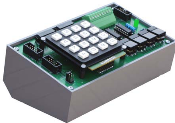
Fig. 4 The keypad/input module 10b can accommodate keypads with 12 or 16 keys. Additionally, eight inputs from outside can be attached.
