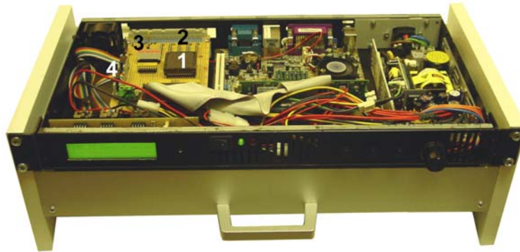
Fig. 1. A low-cost industrial PC based on a Mini-ITX motherboard. 1 - CPLD containing the ATA i/o adapter circuitry; 2 - interface connector; 3 - diagnostic LEDs; 4 - front-panel I/O attachment.
